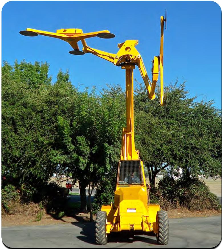
The front suspension combined with the "walking beam" rear axle of the HDR1100N-H provides a stable ride over berms when cross hedging. The narrow power unit and cutting arms provide for efficient hedging in the tightest planted orchards
