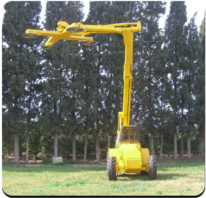
The center pivot of the boom allows for a flat topping height of up to 24 feet.
