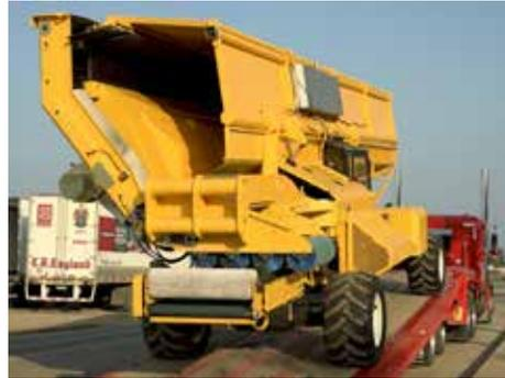
4-wheel steering allows the **Twin D T4 Shaker** to perform tight turns and fit well into commonly planted orchards.
